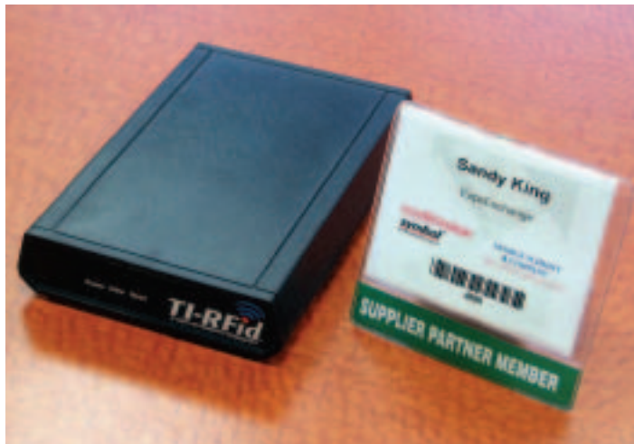
RFID is made up of two basic component parts—the tag, which can be incorporated into a name badge, and the reader, which is about the size of a small pizza box.
